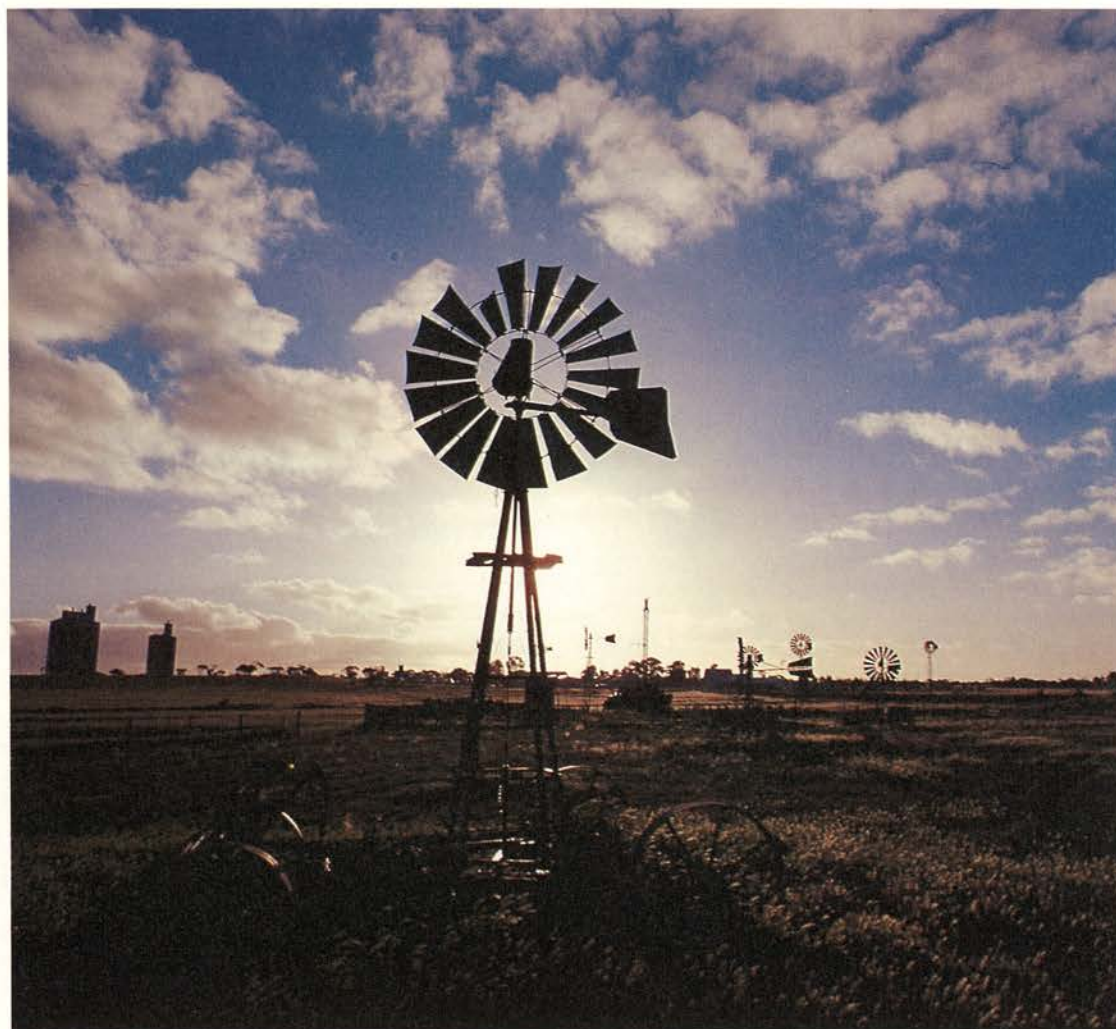
Windmills for pumping artesian water are common in rural areas. These are in Penong, SA. Photograph by Reg Morrison.
